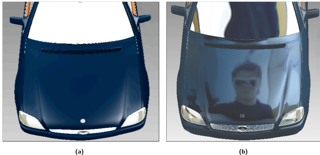
Figure 5.11: A scene containing a virtual car model (a) without and (b) with virtual reflections.
