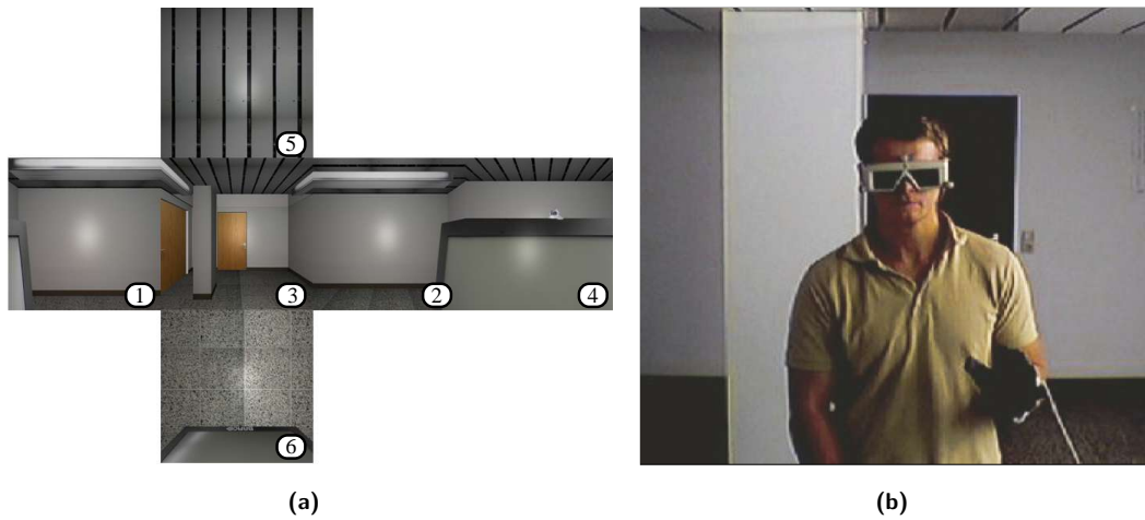
Figure 5.9: (a) Cubic environment map of the synthetically generated model of a responsive workbench of the VR laboratory and (b) the image, grabbed with the USB camera on top of the responsive workbench, to be exchanged with the front texture (3).
