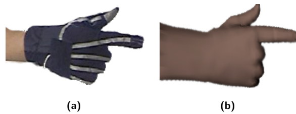
Figure 5.10: Mapping between real and virtual input devices: (a) pinch glove and (b) virtual model.
