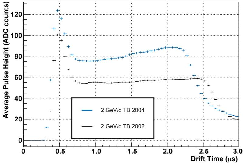
**Figure 7.28:** Average pulse height of pions at 2 GeV/c in chamber2 in 2002 (black) and 2004(blue). While the maximum drift time is at the nominal value of  $2\ \mu\text{s}$  for 2002 data, the maximum drift time in 2004 is smaller ( $\approx 1.6\ \mu\text{s}$ ).
