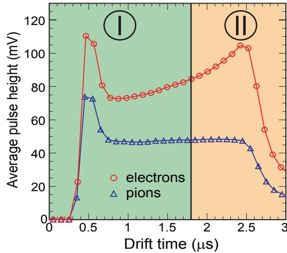
**Figure 6.8:** Illustration of the two-dimensional likelihood method. The chamber is subdivided into two sectors. In sector II transition radiation is preferably absorbed. The measurement of deposited charge in sector I additionally helps to discriminate electrons from pions.
