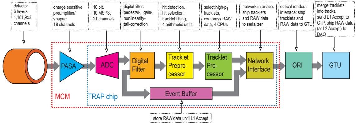
**Figure 4.14:** Schematic overview of the readout electronics [Aam08].
