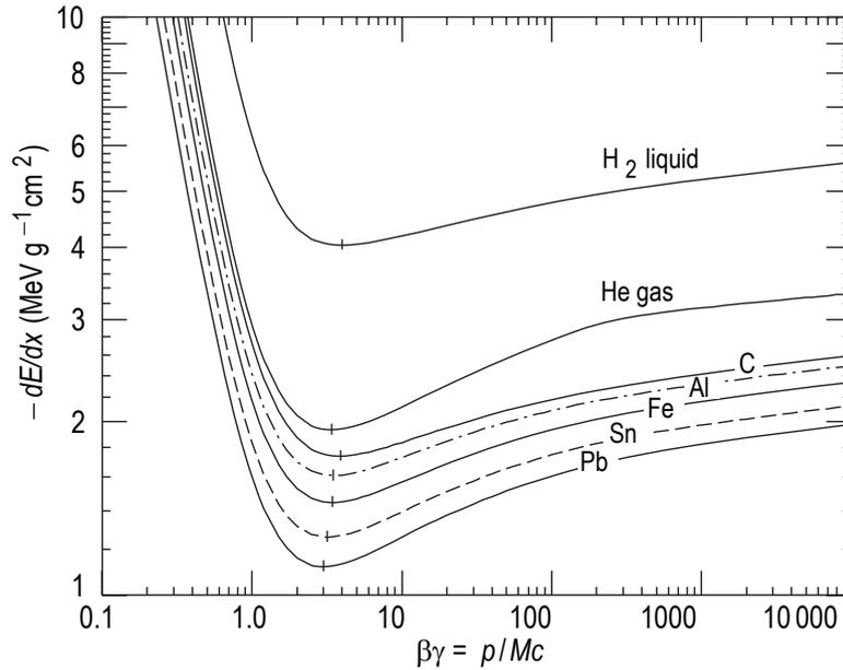
**Figure 4.4:** Calculated mean energy loss of pions in different materials. Taken into account is only the energy loss by ionization. The curve follows the *Bethe-Bloch Formula* [Ams08].
