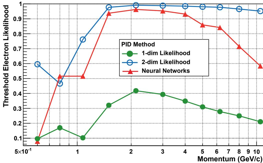
**Figure 8.5:** Threshold for 90% electron efficiency versus momentum for neural networks (red triangles), 1-dim likelihood (green dots, and 2-dim likelihood (blue circles).
