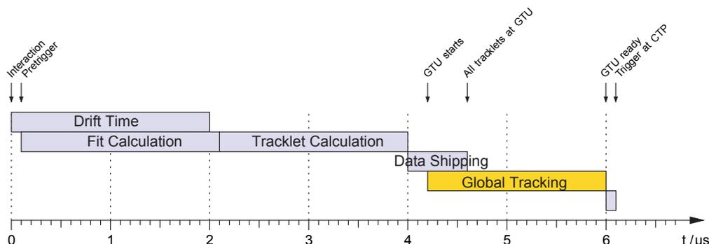
**Figure 9.5:** Trigger timing for the TRD [dC03].
