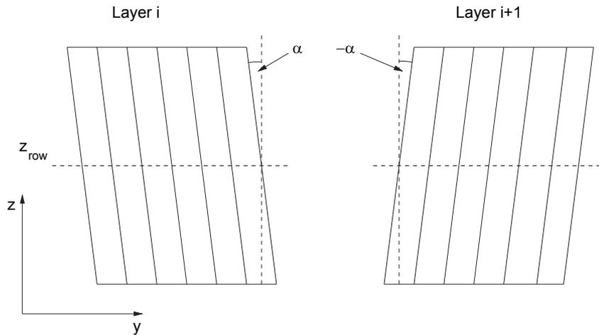
**Figure 4.16:** In order to improve the position resolution in direction of the long side of the pads ( $z$  direction) the readout pads are tilted by an angle  $\alpha$ . The direction of the tilt angle is changed in consecutive layers [TRD01].
