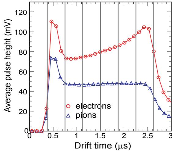
**Figure 6.10:** Illustration of the input for the artificial neural networks using the deposited charge in eight slices of a TRD module. Analogous to the two-dimensional likelihood method on deposited charge the chamber is divided into several slices.
