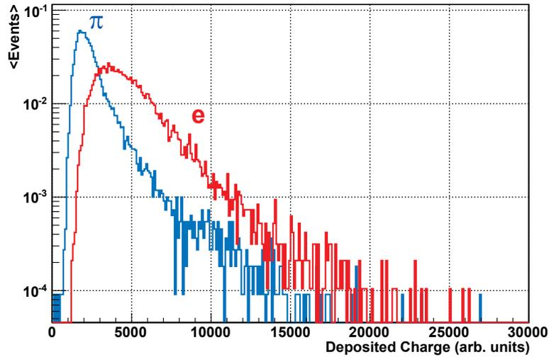
**Figure 7.5:** Total deposited charge for particles with a momentum of 2 GeV/c. Electrons are shown in red, pions in blue.
