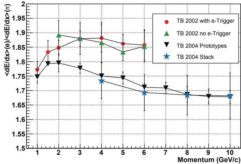
**Figure 7.26:** Ratio of the mean deposited charge for electrons and pions versus momentum. Ratios for 2002 data (with electron trigger (red dots) and without electron trigger (green triangles)) and 2004 data (prototypes (black triangles) and stack (blue stars)) are shown. The plotted ratios are the average values for all the chambers used in the run.
