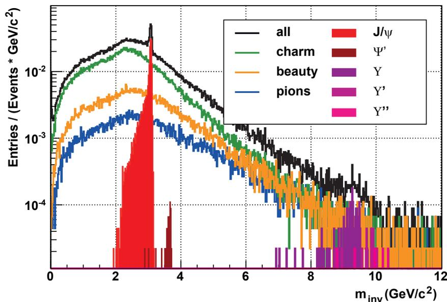
**Figure 9.16:** Invariant mass spectrum of dielectrons using the likelihood on total deposited charge (black curve). The spectrum is normalized to one event and a bin width of  $1 \text{ GeV}/c^2$ . The different contributions to the spectrum are also shown. The signals originating from quarkonia are plotted in full color, contributions to the background as lines. Only the contribution of pions can be reduced by particle identification.
