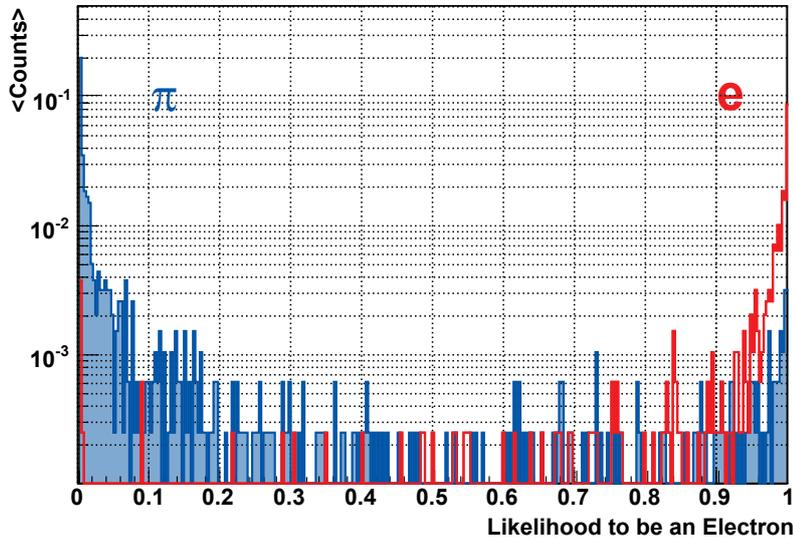
**Figure 7.19:** Likelihood distribution of electrons (red) and pions (blue) with a nominal momentum of 2 GeV/c. A large contamination of pions at large electron likelihoods is clearly visible.
