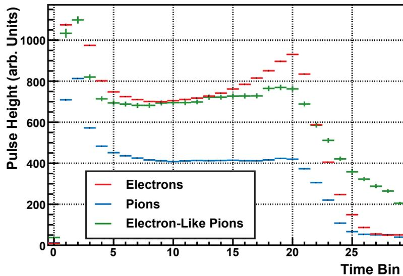
**Figure 7.21:** Average pulse height distributions for electrons (red), pions (blue), and pions with an electron likelihood larger than 0.99 (green). Pions with large electron likelihood show in contrast to the other particle classes a clear signal at time bins larger than 24.
