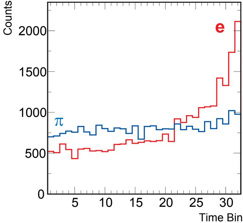
**Figure 6.7:** Time bin with the largest amount of charge for electrons (red) and pions (blue) in the drift region. The momentum was 1 GeV/c [And01].
