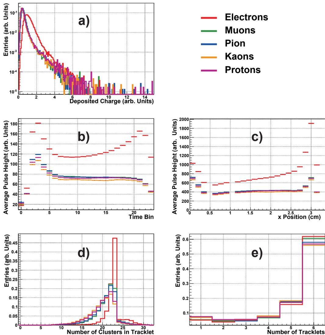
**Figure 8.2:** Monitoring plots of the AliTRDcheckPID task. The plots are shown for electrons (red), muons (green), pions (blue), kaons (orange), and protons (purple) with a momentum of  $2 \text{ GeV}/c$ . The plots are **a)** the deposited charge per tracklet, **b)** average pulse height versus time bin, **c)** corrected average pulse height versus  $x$  position, **d)** number of clusters per tracklet, and **e)** number of tracklets per track.
