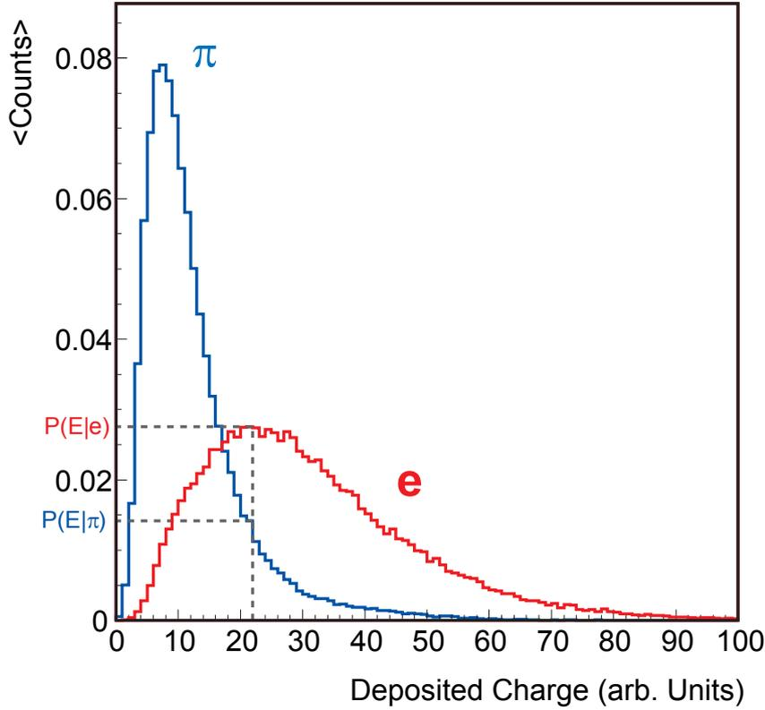
**Figure 6.6:** Deposited charge for electrons (red) and pions (blue) in one TRD module. This data was taken during the test beam of 2002. The momentum of the particles was  $2 \text{ GeV}/c$ .
