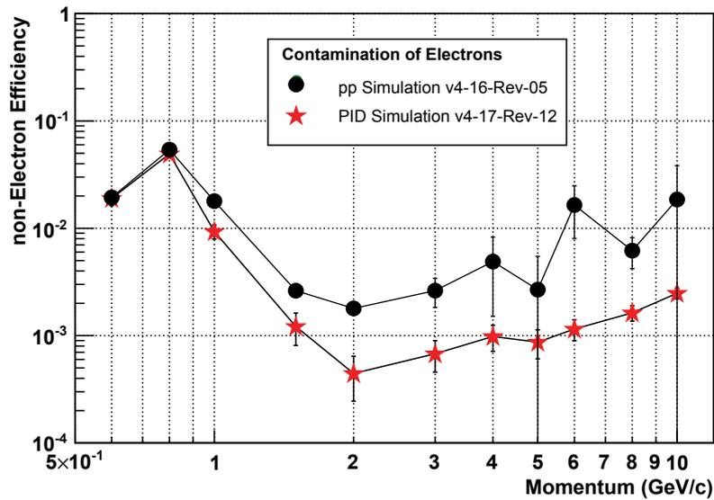
**Figure 8.9:** Non-electron efficiency versus momentum for artificial neural networks. The results of a direct calculation (black dots) and of an indirect estimation using the momentum dependent multiplicities (red stars) are shown. For details refer to the text.
