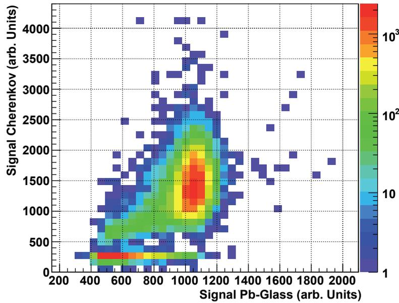
**Figure 7.20:** Correlation plot for Pb-glass and Cherenkov detector for 2 GeV/c data. Contrary to the correlation plots of 2002's beam time (Figure 7.3), a fraction of particles with a high Cherenkov signal but small energy deposition in the Pb-glass can be seen.
