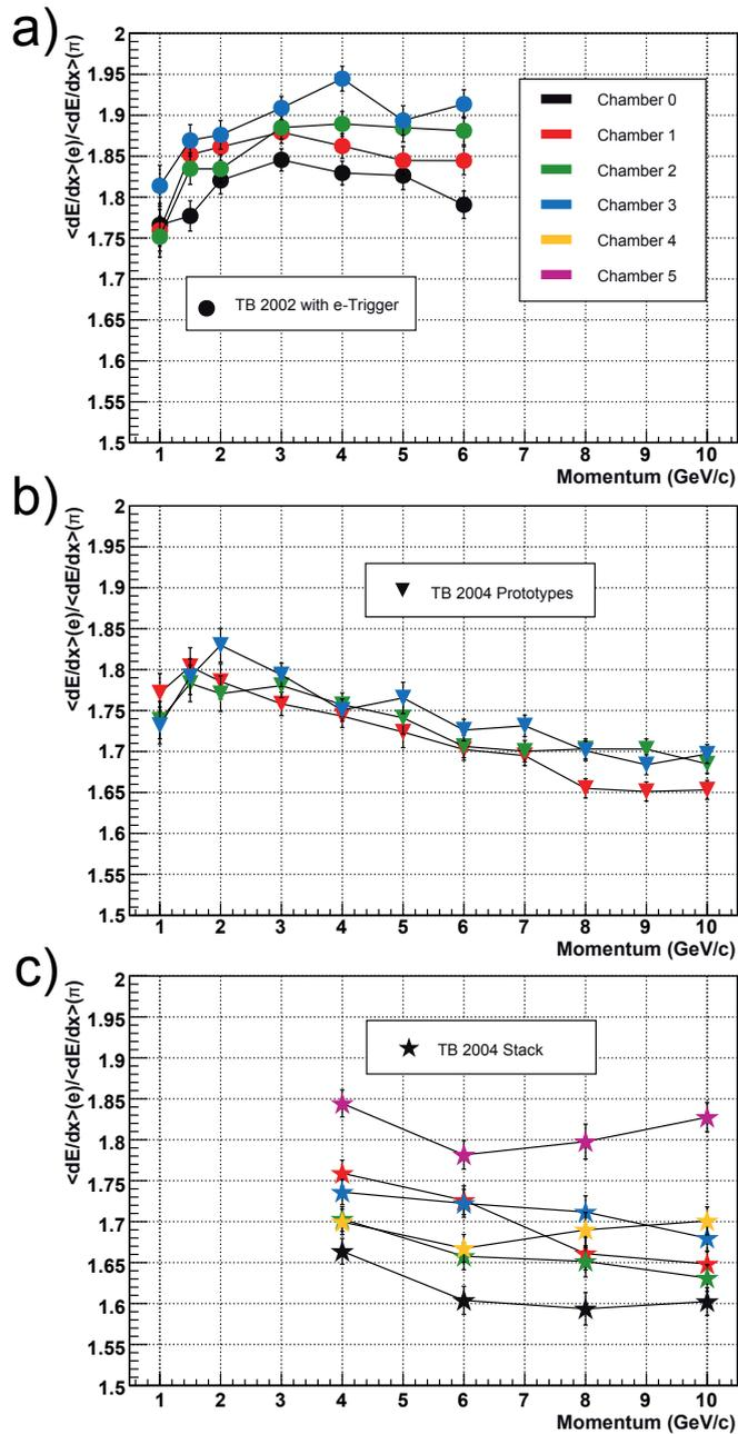
**Figure 7.27:** Ratio of the mean deposited charge for electrons and pions versus momentum in each TRD chamber. Ratios for **a)** 2002 data (with electron trigger (dots)), **b)** 2004 prototypes tests (triangles), and **a)** stack measurements (stars) are shown.
