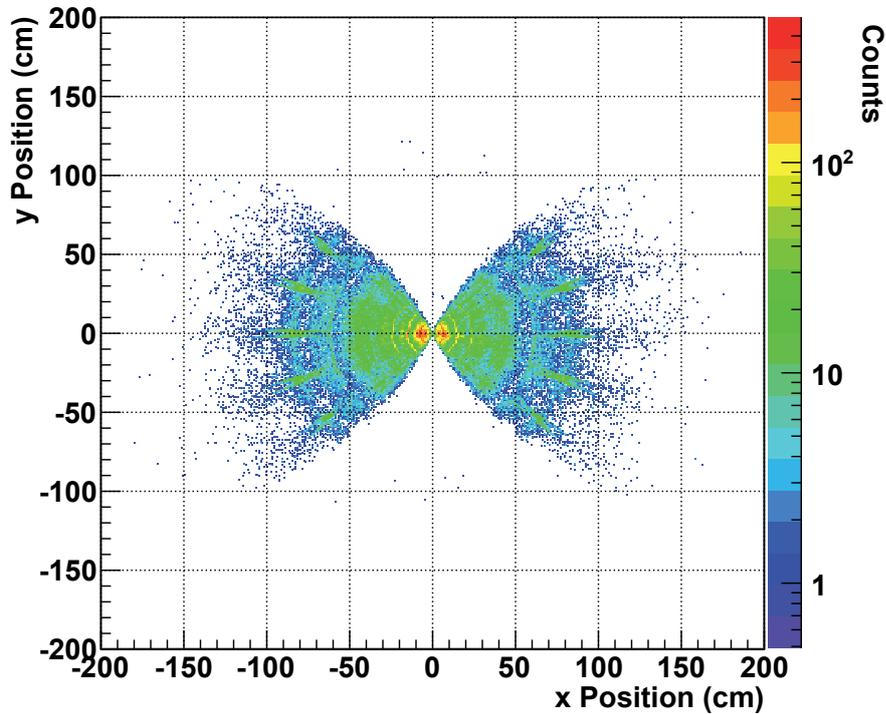
**Figure 9.3:** Conversions in ALICE for 32 million  $pp$  collisions at 10 TeV/c [Hei09]. All conversion points are shown where at least one track can be reconstructed in the Transition Radiation Detector. In this simulation eight TRD Supermodules were active. Since photon conversions occur preferably in material with a high nuclear charge  $Z$ , the layers of the ALICE Inner Tracking System as well as the inner part of the Time Projection Chamber can be seen.
