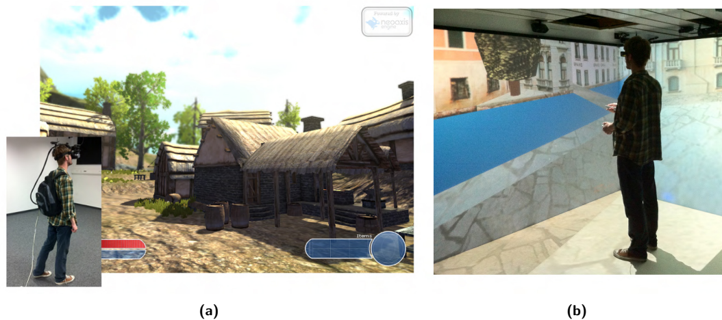
Figure 6.3: Examples of student projects using VINS. (a) A Demo of the NeoAxis game engine updated to work with HMD and optical head tracking. (b) City visualization rendered with the IrrLicht engine in our 3-Wall CAVE. Nintendo's Wii controller is used for navigation and the user's head position is tracked with Kinect (not in the picture).
