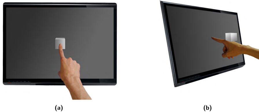
Figure 2.2: Illustration of the occlusion problem; while the occlusion cues (a) indicate that the user’s finger is in front of an object, binocular disparity cues (b) are suggesting that the user’s finger is behind the object.
