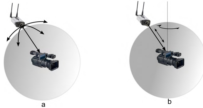
Figure 5.3: Illustration of the WIM interaction: a) Single finger pan gestures map to azimuth and elevation of a virtual trackball control centered on the user's current position. b) Pinch and rotate gestures define scaling and rotation around the main-camera's up-axis.
