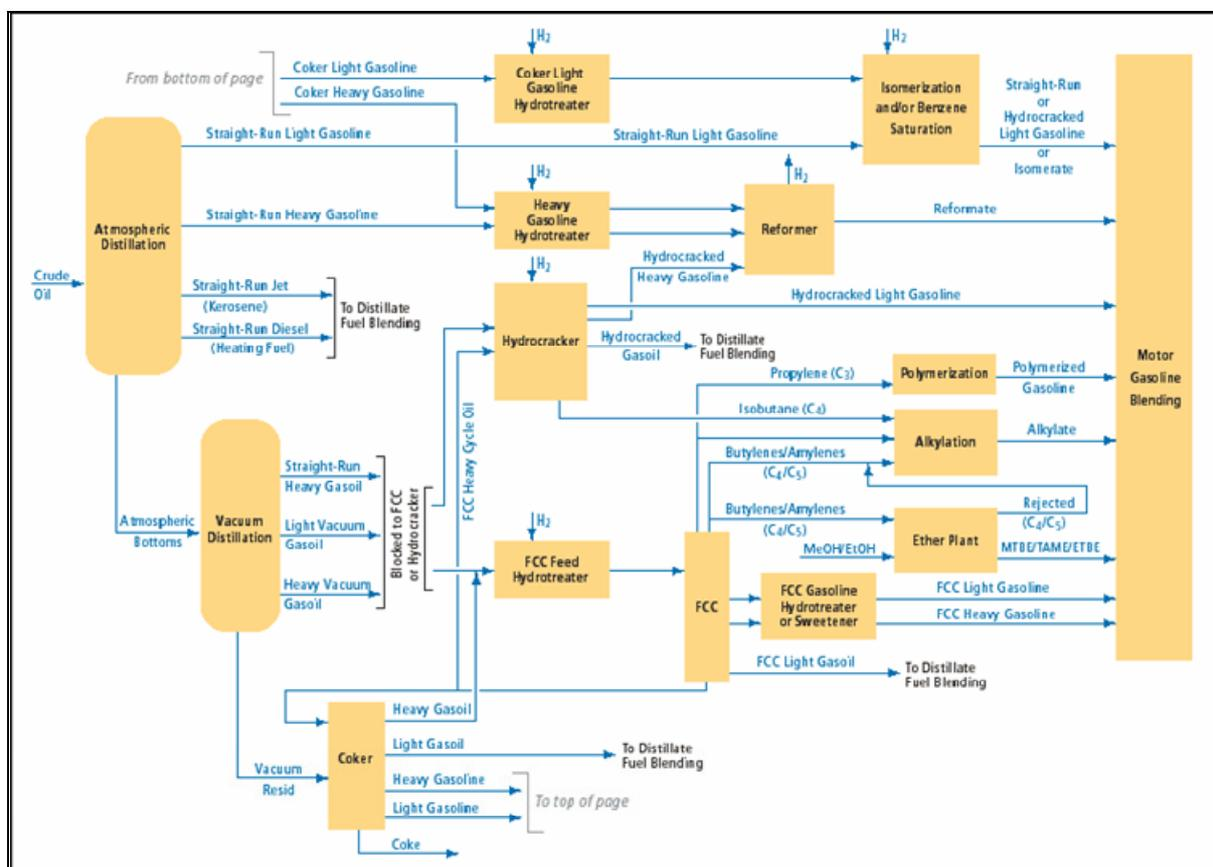
Figure 2.8 Schematic overview of the industrial refining process [10].
