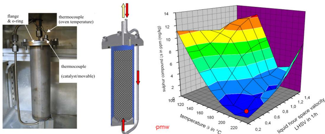
Figure 3.3 Picture along with schematic design of the adsorptive reactor used at the OWI, Aachen (left) and a graph illustrating the dependance of the sulfur removal on the process parameters during desulfurization of the heating oil EL-series [51] (right).
