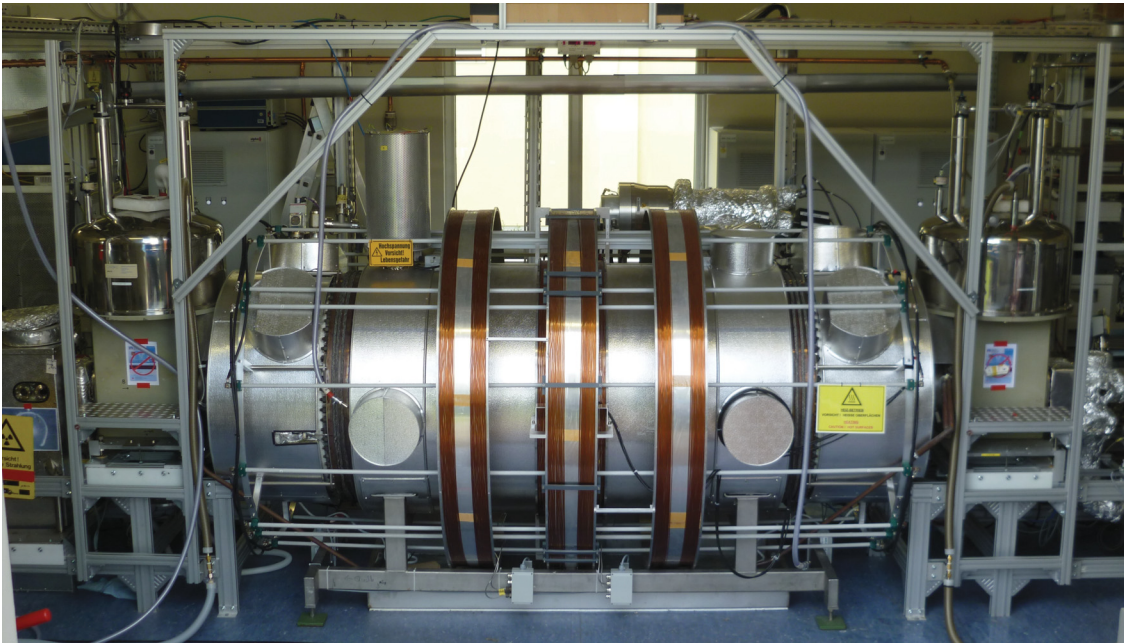
Figure 51: Set-up of the monitor spectrometer. Source chamber and source magnet are on the left side. Detector magnet and chamber on the right side. The four air coils surrounding the spectrometer (the fourth coil is inside the outer coil in the middle of the spectrometer) are visible in the central area.
