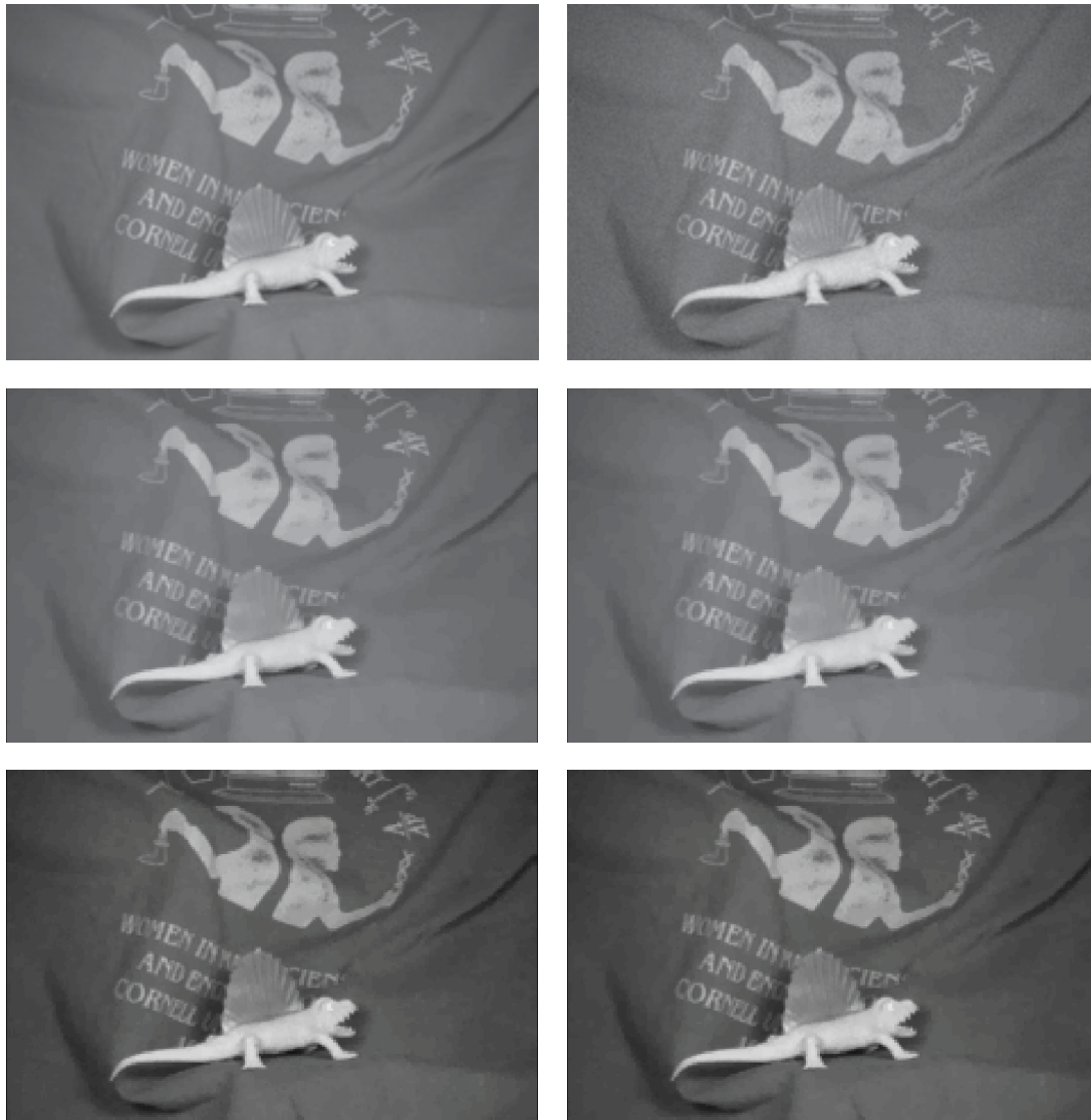
Figure 5.4.: Reconstructed images generated by the joint models. Top-left: ground truth image, top-right: noisy image, middle-Left: TV - L^2 optical flow, middle-right: TV - L^2 mass preservation, bottom-left: TV - TV optical flow, bottom-right: TV - TV mass preservation.
