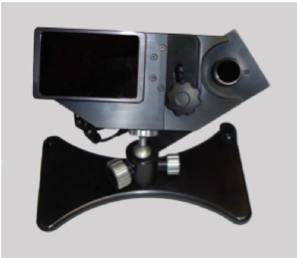
Figure 2: Desktop mounted EyeLink 1000 system used for gaze recording. The EyeLink 1000 camera and the infrared illuminator was placed just below the computer monitor where the experimental stimuli were presented.
