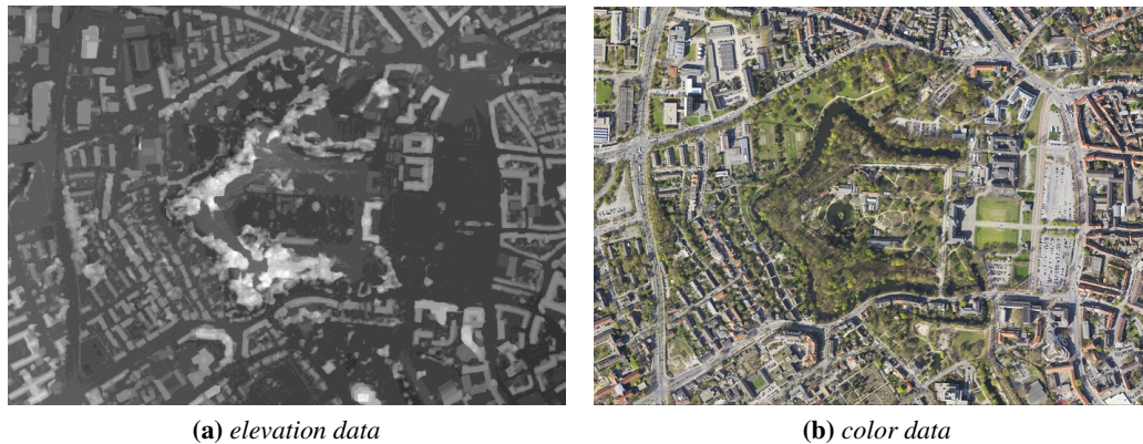
Figure 1.1: A visualization of two kinds of DSM data which are represented as two 2D arrays. The elevation data (left) are also called height map in which brighter areas are more elevated than darker ones.
