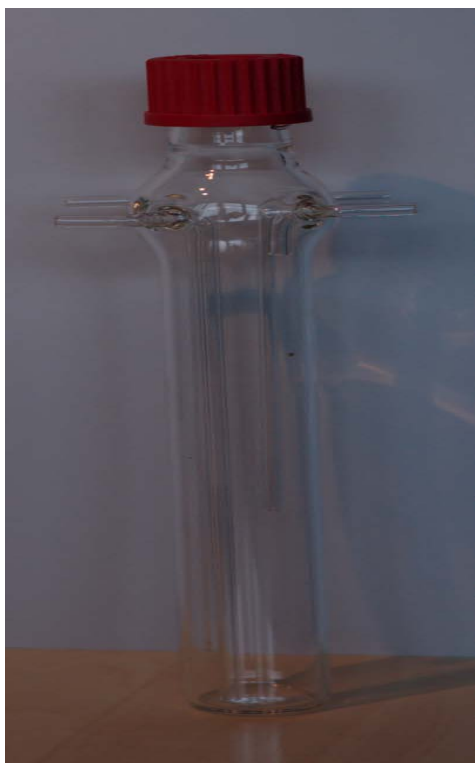
Figure 3.7: Picture of a bioreactor The bioreactors used as culture vessels for the continuous cultures were custom made
