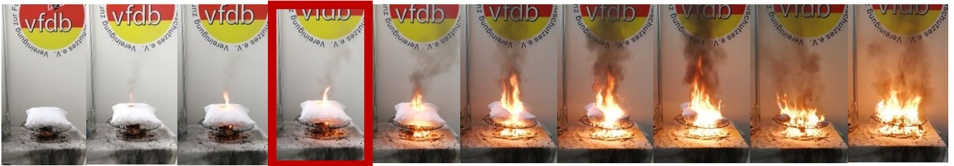
Figure 4. Time course (90 seconds) for a small burning pillow. The time interval between each picture is about 10 seconds. The alarm sounded when the fire size was similar to the size of the fire in the framed image.
