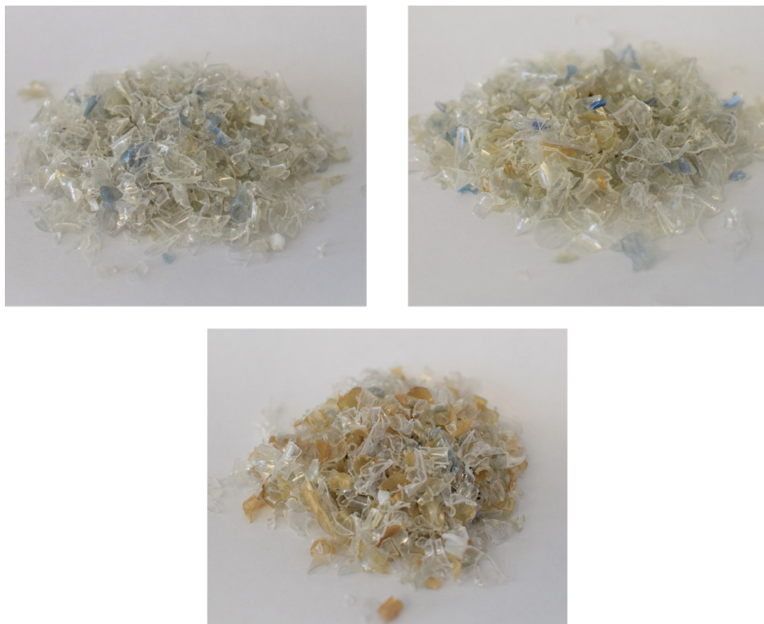
Figure 3 Samples of clear PET flakes after roast test (top left: no coated bottled included, top right: current deposit return scheme material, bottom: material quality expected for 2022).
