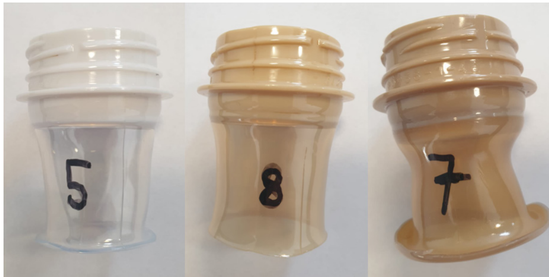
Figure 2 Bottle necks after thermal load with differing results.
