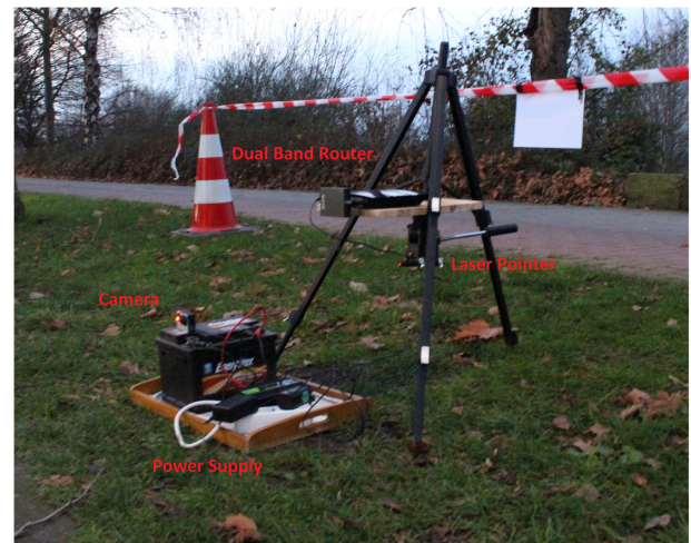
FIGURE 2. A picture of the system's sending unit. The different hardware components (Router, laser pointer, camera and power supply) are labeled.
