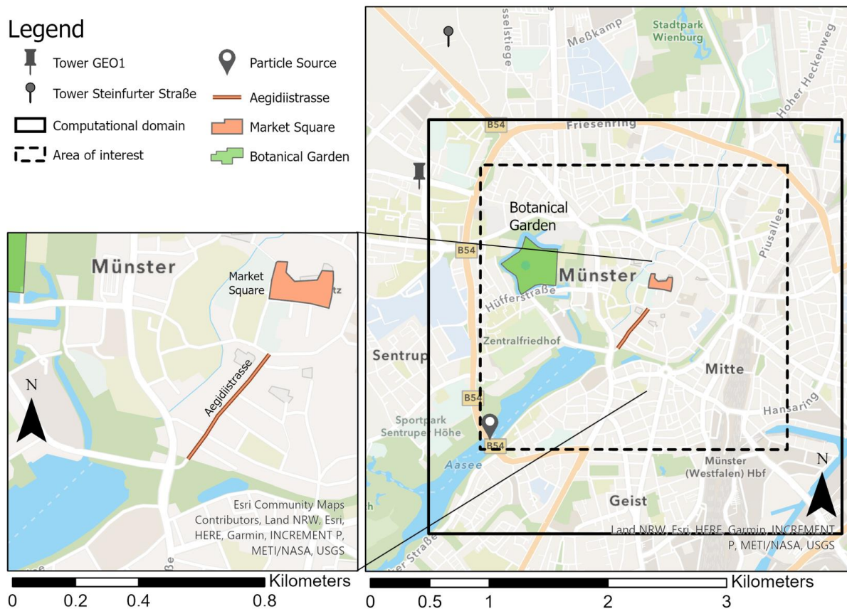
Figure 1. Map of Münster with meteorological measurement towers next to “Steinfurter Straße” and on the rooftop of GEO1. Topography data for the computational domain area were used as input for the simulation software PALM. Simulation results for the area of interest were analyzed.
